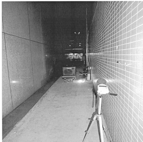
FIG. 13. Experimental setup in a 1.55-m-wide street canyon for outdoor measurements.
