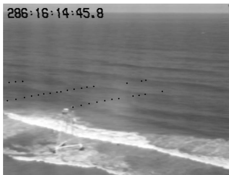
FIG. 4. Video image of CRAB during one of its daily bathymetry measurement excursions. The position of the GPS antenna mounted aboard the CRAB was used as a ground control point (GCP) during the photogrammetric transformations. The position of the antenna within successive images (indicated by black dots) served as multiple GCPs necessary for accurate transformations.
