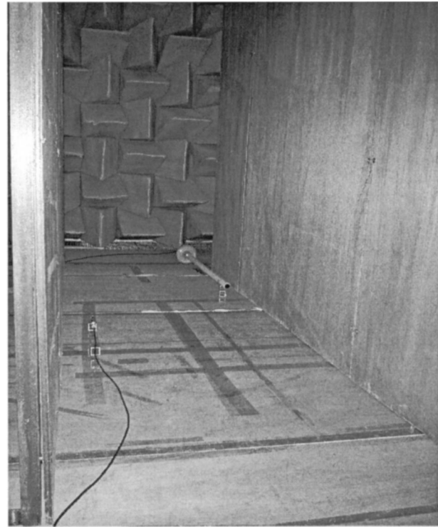
FIG. 7. A 1:10 scale model set up in an anechoic chamber for measurement of sound propagation in a street canyon.
